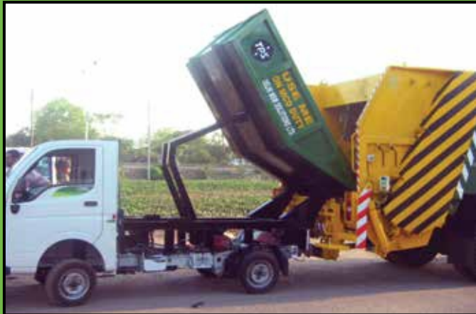
Tipper discharging garbage into garbage compactor
