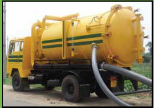
Suction Dump Tank with cyclone for collection of suctioned silt.
