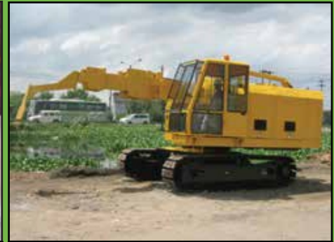
Furnace Tending & De-bricking Machine
