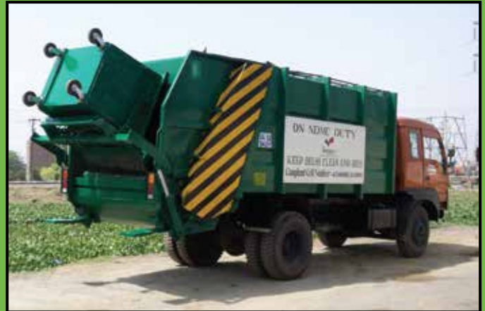
1100 Ltr Bin being unloaded in TPS Compactor
