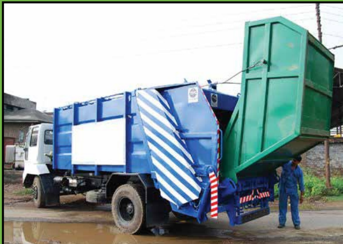
3.5M bin being lifted into Garbage Compactor
