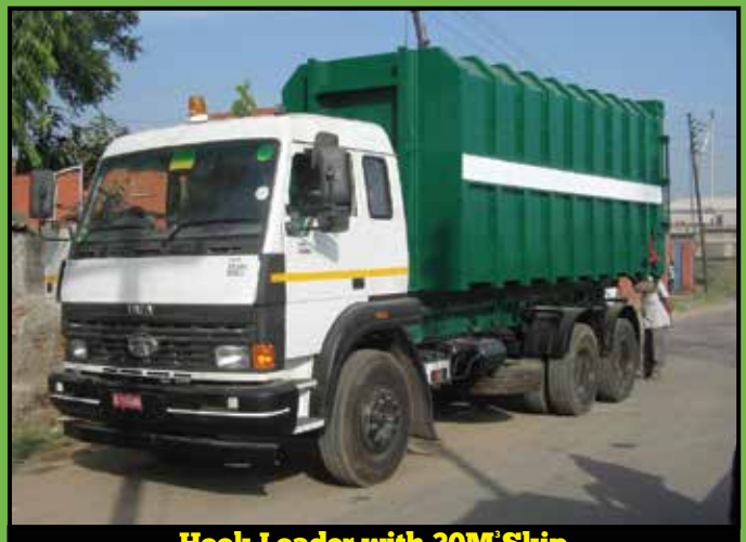
Hook Loader with 20M 3 Skip
