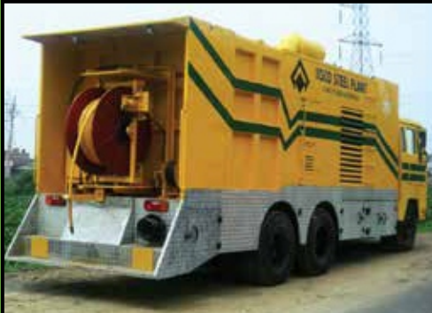
De-silting Machine for Cleaning of Trunk Sewer Pipeline
